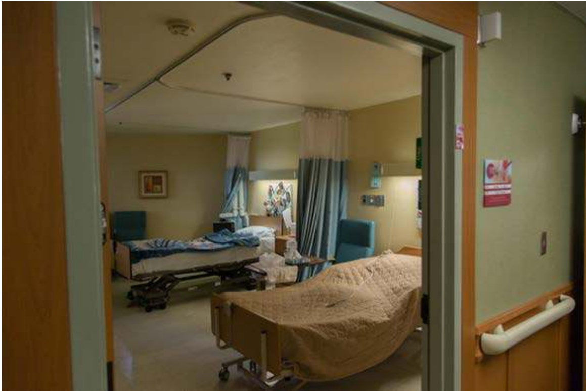
Figure 6: Incumbent fluorescent lighting in the double resident room. The single room had a similar wall-mounted luminaire above the bed as the only lighting in the room.
