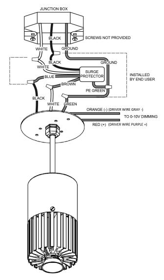
Fixture comes with 5 wire conductors
