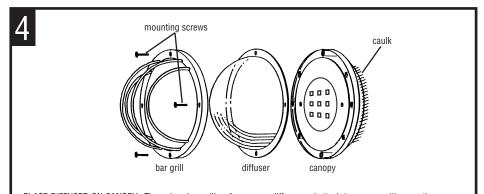
PLACE DIFFUSER ON CANOPY. Then place bar grill or frame over diffuser and attach to canopy with mounting screws. (8-32x1/2, 4 combination head screws provided)
