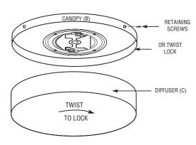
Attach diffuser and secure in place with diffuser retaining screws.
